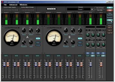
Click this button to open the Compressor window for the A and B outputs. Each compressor has five knobs: Attack, Release, Threshold, Ratio, and Output. Click and drag on the individual knobs to adjust each parameter. An analog-style meter indicates the amount of compression applied in decibels.
